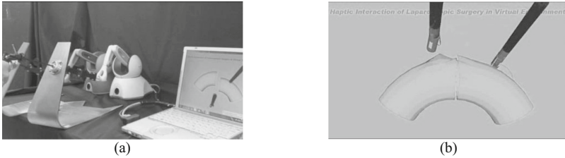
Fig. 1. The (a) physical and (b) graphical interface of our VR training system.
