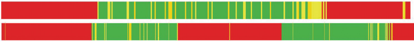
Fig. 1. Quality analysis for two recordings with a binocular eye-tracker. The color represents measurement errors (red), successful tracking of both eyes (green) and of only one eye (yellow) over time. It is easy to visually assess the overall quality of a recording as well as the nature of individual tracking failures (Color figure online).
