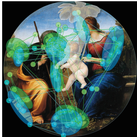
Fig. 4. Simultaneous overlay of multiple visualization techniques for one scanpath of an image viewing task. The background image is shown together with a scanpath representation of fixed-size fixation markers (small circles) and generated fixation clusters (bigger ellipses) for left (green) and right (blue) eye. AOIs were annotated by hand (marked as white overlay) (Color figure online).
