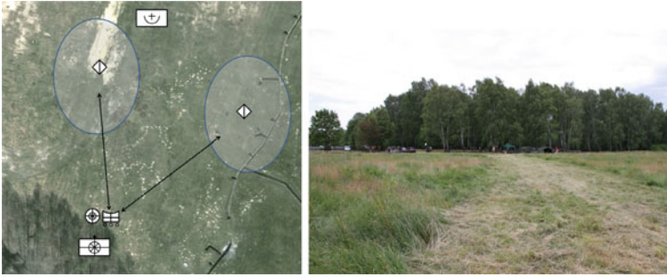
Fig. 1 The MedEvac scenario in an overview: Starting from the marked position on the bottom left corner , the participants have to go to each of the marked way-points and search the area for the dummy. After locating the dummy and acquiring a GPS coordinate of it, the robot is supposed to bring the dummy back to the starting position. The whole scenario takes place in a 150\text{ m} \times 150\text{ m} area with a distance from the dummies to the controller's tent of about 75 m
