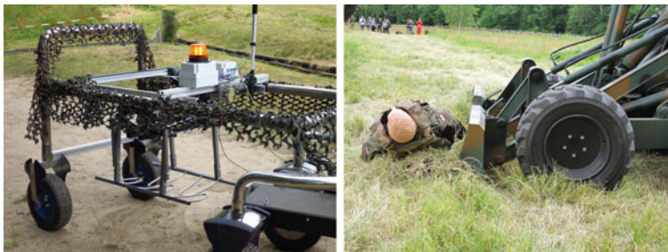
Fig. 4 Two teams presented lifting strategies without using a robot arm. While the University of Oulu constructed a lifting mechanism, team Marek used sheer force in form of a large fork lifter
