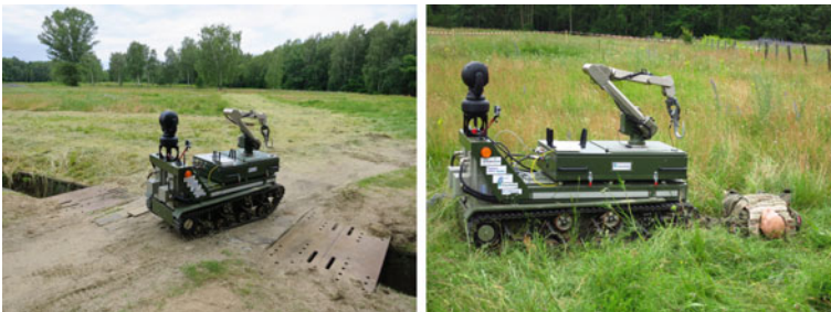
Fig. 5 Left The FKIE robot at the starting position. Here the dummy had to be brought back to. Right The robot arriving at the first dummy. From here the manipulation task was to hook up the gear
