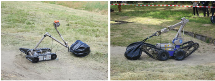
Fig. 3 Two other competitors using a similar strategy to our approach: towing the dummy back to the starting point. Due to the size of the robots only the 10 kg dummy ( black bag ) could be moved
