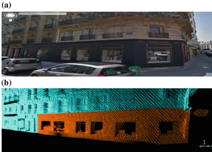
Fig. 8 a Google street map view photo of the building on Rue Madame with a strong variation of paint color. b Segmentation results of the super-voxel based method
