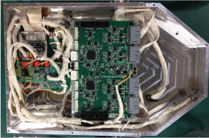
Fig. 9 Moonraker's internal components, with complex wiring harness
