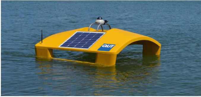
Fig. 2 One of the autonomous surface vehicles from the Inference system. The navigation sensors, computing and batteries are located underneath the two solar panels. The scientific payload is attached to the moon-pool opening underneath the camera. Note the pan-tilt dome camera visible was not used in this study, only the smaller USB camera directly in front of it
