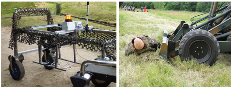
Fig. 4 Two teams presented lifting strategies without using a robot arm. While the University of Oulu constructed a lifting mechanism, team Marek used sheer force in form of a large fork lifter
