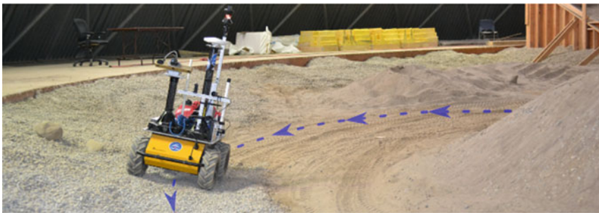
Fig. 1 Our field robot during a 140 m autonomous traverse in the UTIAS MarsDome indoor rover testing environment, with the path overlaid for illustration. In order to compare the performance of stereo and monocular VT&R with the same hardware, we equipped our rover with a stereo camera and used only the left image stream for our monocular traverses
