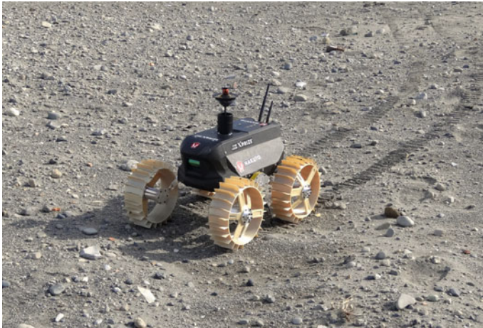
Fig. 3 Moonraker maneuvering in a rocky area. A Leica 360° prism, used for ground truth measurements, is visible on top of the mirror
