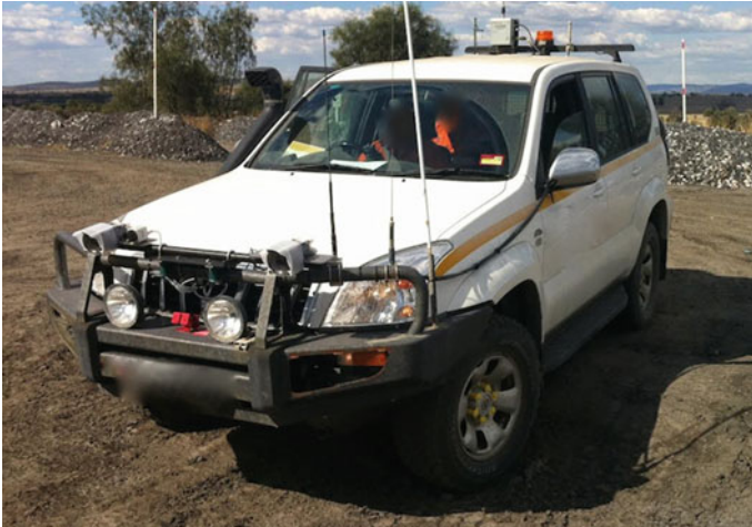
Fig. 4 The experimental dataset gathering vehicle with cameras mounted to the bullbar. Note all images used in this paper were captured from the camera on the left hand side of the vehicle
