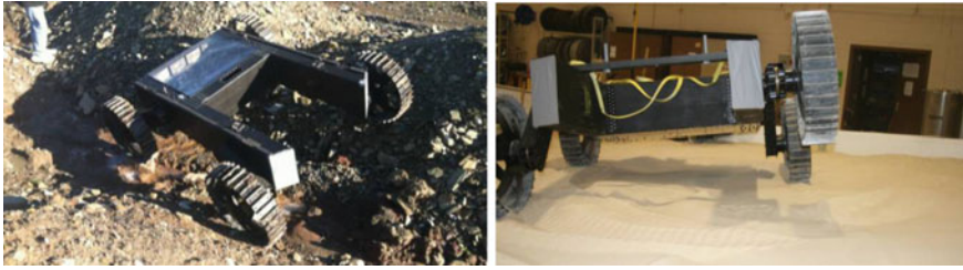
Fig. 6 Field tests ( left ) led to the discovery and study of suspension lift-off ( right )
