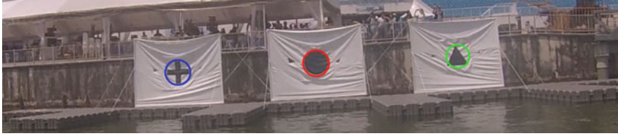
Fig. 5 Placard feature detection. The three correctly detected placards are circled in blue, red, and green
