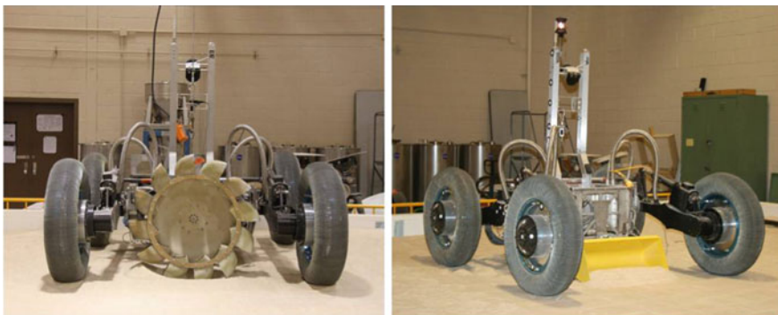
Fig. 1 A robotic excavator configured for continuous ( left ) and discrete excavation ( right )
