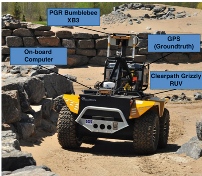
Fig. 3 Grizzly Robotic Vehicle autonomously repeating a route during the CSA field trials, with applicable sensors highlighted. Credit [16]
