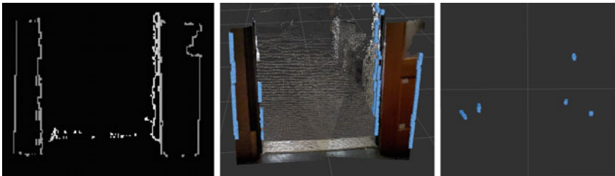
Fig. 4 Left Edge image of doorway. Center Edge pixels identified in the scene. Right Top down view of door edge coordinates
