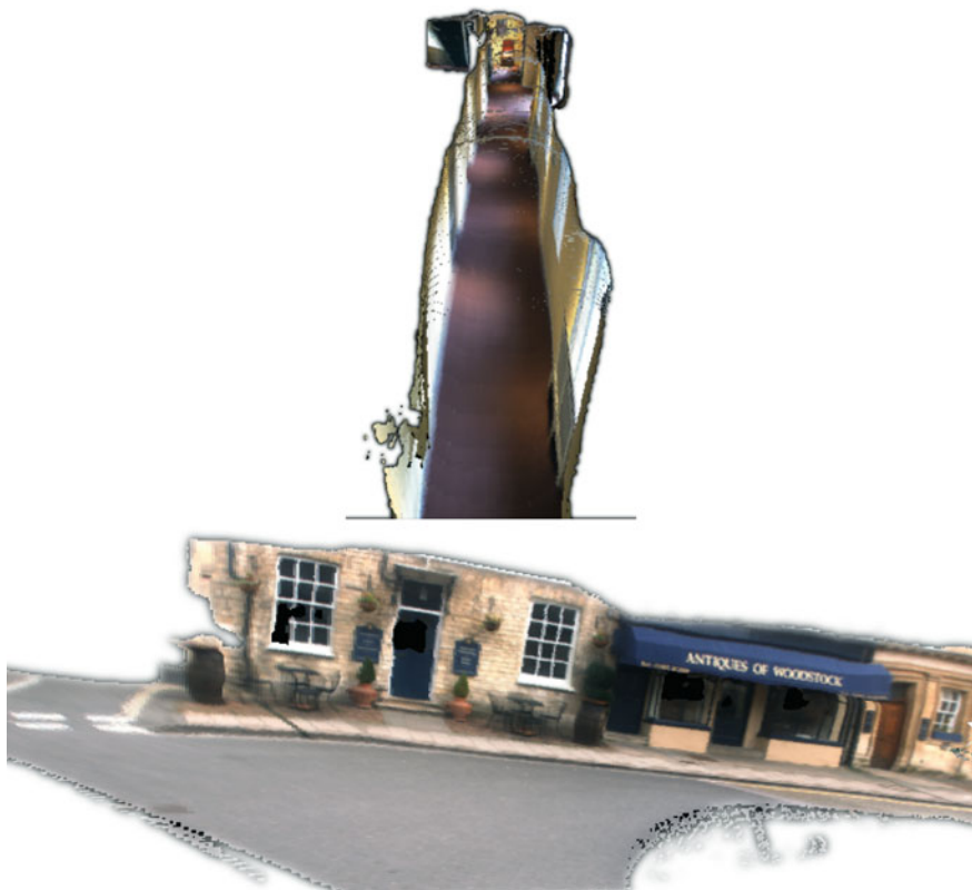
Fig. 6 The final 3D reconstruction of the large scale experiments using BOR 2 G with the Acland building ( left ) and Woodstock, UK ( right )
