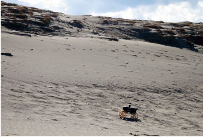
Fig. 2 Moonraker climbs a 10^\circ slope at the Nakatajima Sand Dunes
