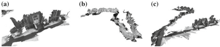
Fig. 11 An example of the reconstruction result for an outdoor snow scene from approximate 5000 stereo frames (final mesh includes approx. 32 million vertices). a A close look at a house in the scene. b An overview of the scene mesh. c An overview of the scene texture
