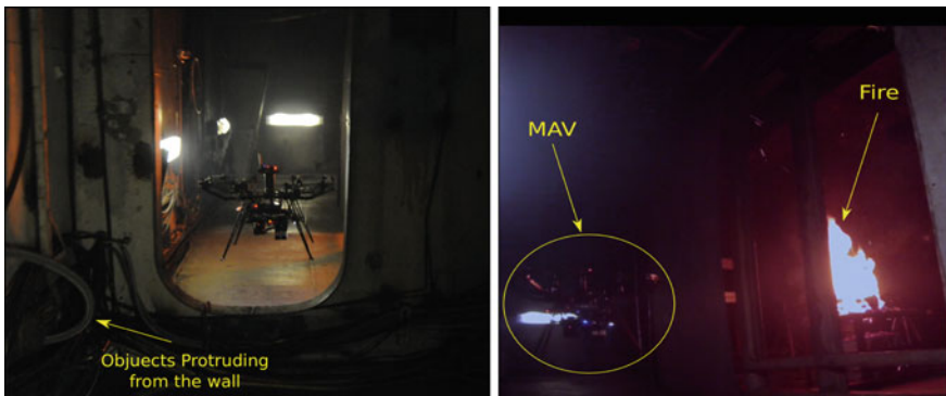
Fig. 1 Autonomous MAV for fire-detection inside a ship: The left picture shows MAV's autonomous flight through doorways. The right picture shows a testing scenario with fire
