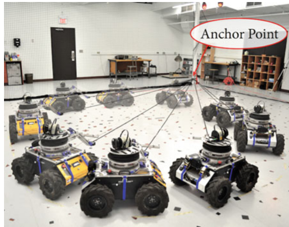
Fig. 10 A time-lapse of the Vicon test shows TReX performing tension-based tether management. Throughout two traverses, the tether was taut with minimal sag
