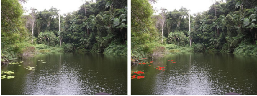
Fig. 6 Example of image segmentation from the ASV for detecting on-water obstacles such as water lilies ( Left original image. Right image with detected obstacles highlighted in red)
