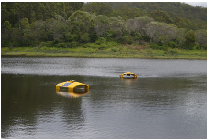
Fig. 7 The two ASVs at the start of a sampling campaign on Gold Creek Dam, Queensland. The retracted gas sampling unit is visible underneath the ASV on the right
