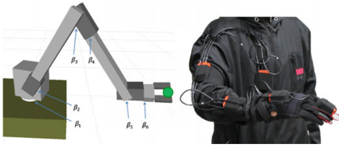
Fig. 2 Directly coupled man-manipulator control. Using several IMUs ( right ) the operator's movement is measured and transferred to the manipulator ( left )
