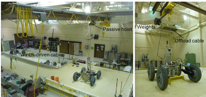
Fig. 2 Gravity offload testing with bucket-wheel ( left ) and front-loader bucket ( right ) on the Scarab robot. A cable pulls up on the robot, tensioned by weights acting through a 2:1 lever arm. The offload assembly hangs from a hoist that is pulled along a rail by a separate winch-driven cable
