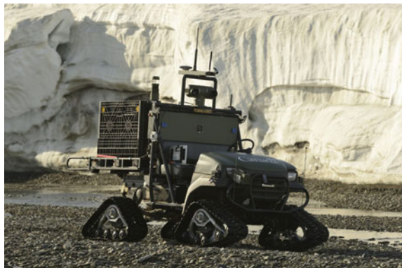
Fig. 1 Multi-Agent Tactical Sentry (MATS) vehicle performing autonomous path following in Alert (Nunavut, Canada). Polar environments cause issues for vision-based systems such as ice, snow, and 24-h sunlight with a peak elevation of 12^\circ . This leads to unsatisfactory results for current vision-based systems
