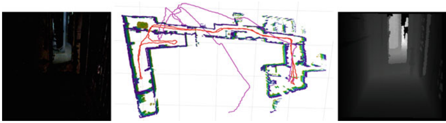
Fig. 5 Localization in degraded visual environment: Pink Odometry, Red Localization. The center plot shows the odometry, localization results with the 3D octomap. Pictures on both sides show the RGB and depth images from onboard RGB-D camera
