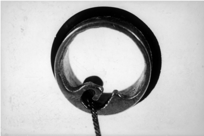
Fig. 3.3. The trip wire, passed via the biopsy channel, is secured into the notch of the inner (ligating) cylinder. Note the elastic “O” ring mounted on the distal end of the ligating cylinder. (From Stiegmann et al. [6], with permission from Elsevier).
