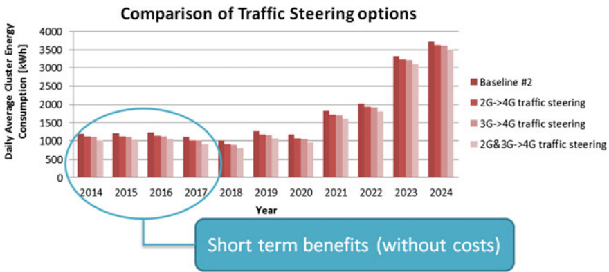
Fig. 18 Performance comparison of energy consumptions obtained by means of different traffic steering options with respect to the baseline system #2 (“Network renewal in 2017”)
