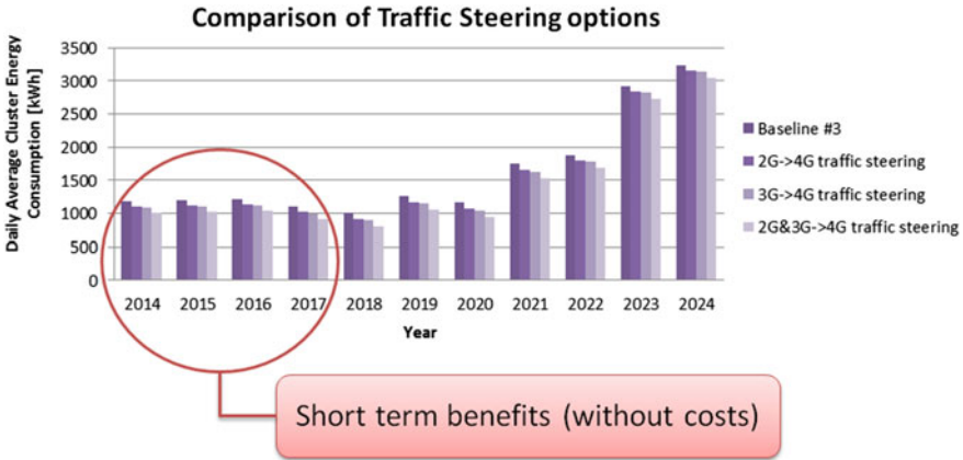
Fig. 19 Performance comparison of energy consumptions obtained by means of different traffic steering options with respect to the baseline system #3 (“Continuous network renewal”)
