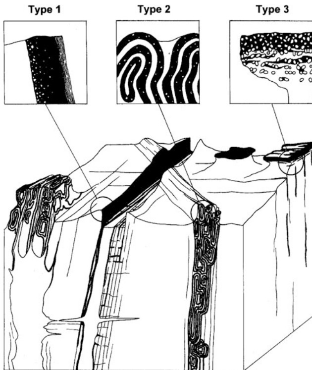
Fig. 13.5 A schematic block-diagram showing the different macro-morphological types of ferruginization in relation to dykes and pipes of volcanic rocks and fracturing of the host sediment in the Kokořín area. Type 1 subvertical planar bodies lining contacts of basaltic dykes or filling joints and faults; Type 2 undulating ferruginous crusts; Type 3 strata-bound subhorizontal bodies. After Adamovič et al. (2001)
