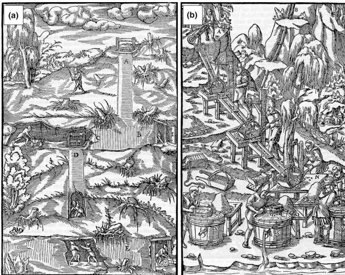
Fig. 10.7 a Depiction of subsurface ore mining and b of placer mining in the famous work De re metallica libri XII (twelve books on mining and metallurgy) by Georgius Agricola, published in 1556
