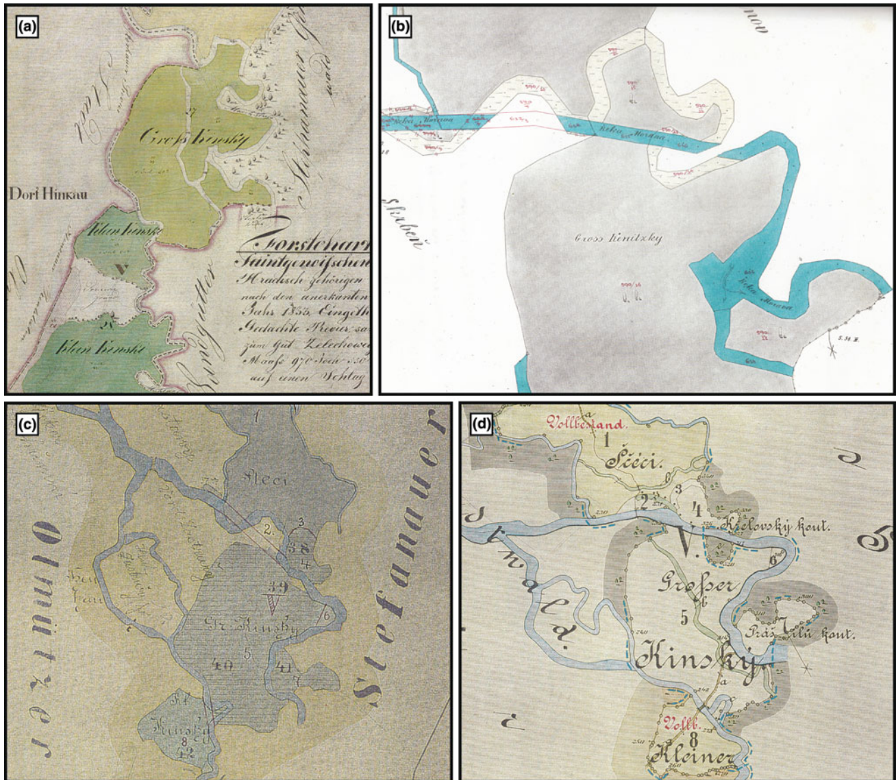
Fig. 23.4 Channel development of the Kenický meander hydrological node in the nineteenth century on old maps. a management map of forest district Štěpánov and Střeň from 1829 (original scale 1:5,200); b cadastral map of the Střeň settlement from 1870 showing the artificial shortening of the Morava channel (original scale 1:2,880);
