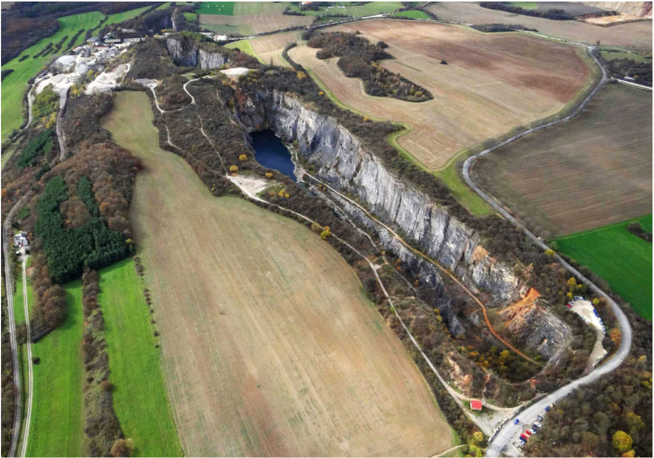
Fig. 6.12 One of the frequently visited hiking trails leads along the rims of deep open-pit limestone quarries near Mořina. This specific style of quarrying was necessitated by the vertical dip of the best quality limestone layers (Photo V. Konvička)
