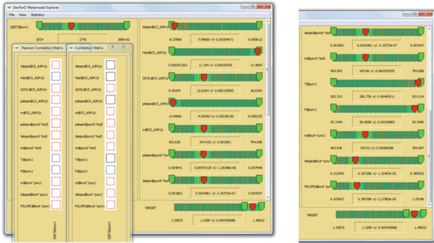
Fig. 5 Example 1, Scenario 1: metamodel and correlations for the parameters and criteria listed in Table 2. Criteria from top to bottom: tslope, Had, QVOL, pslope, m of the compressor, pslope, tslope and m of locE , T and P of junc1 , m, tslope and pslope of locA^junc1
