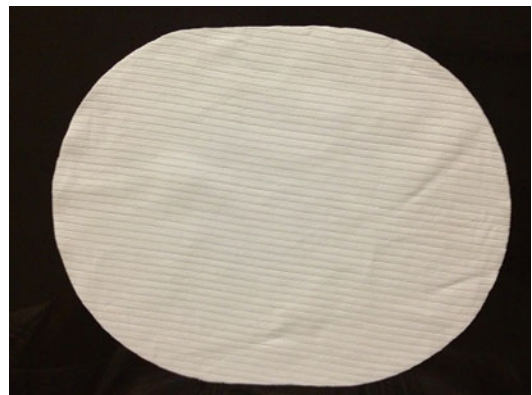
Fig. 6.9 Dual-sided PTFE mesh (microporous)
