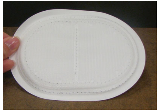
Fig. 6.10 Microporous PTFE and macroporous Polypropylene composite mesh
