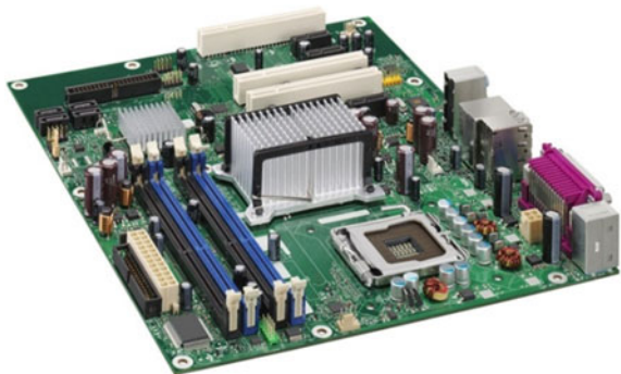
Fig. 2.9 A computer “mother board” is a good example of a PCB
