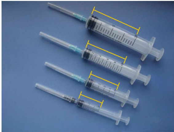
Fig. 11.16 Determining the inner diameters of disposable syringes
