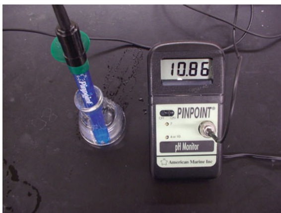
Fig. 10.13 A pH meter with a pH electrode
