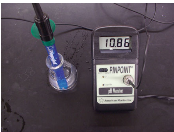
Fig. 10.13 A pH meter with a pH electrode
