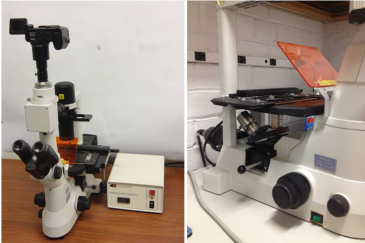
Fig. 9.6 Inverted fluorescence microscope showing the overall shape ( left ) and objective lenses/filter cubes ( right )
