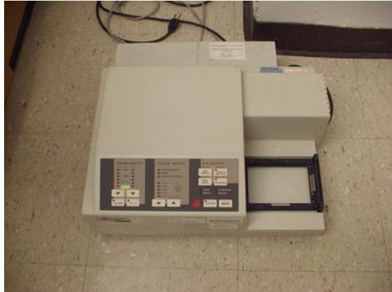
Fig. 13.3 A microplate reader. A microplate is placed onto the bottom right tray and inserted into the reader
