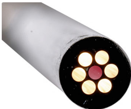
Fig. 8.14 Cut-away view of a reflection probe. The core fiber delivers the incident light, and the shell-side bundle of fibers detects the reflected or backscattered light. Accessed in October 2015 from http://oceanoptics.com/product/premium-grade-reflection-probes . Reprinted with Ocean Optics permission. © Ocean Optics 2015
