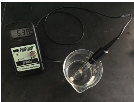
Fig. 1.15 A fluoride ion selective electrode is measuring fluoride concentration from tap water
