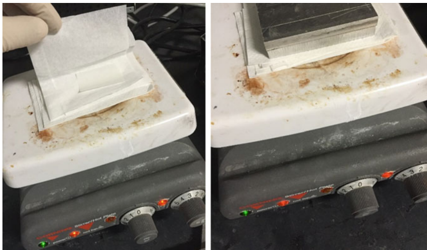
Fig. 14.31 Paper is dried on a hot plate. A weight is placed on the paper
