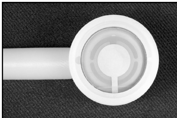
Fig. 11.13 A 5 MHz crystal is placed within the sensor holder of QCM200. In this mode, the QCM can be used as a “balance.” To install a flow cell, the white plastic cap and O-ring should be removed. Accessed in October 2015 from http://www.thinksrs.com/downloads/PDFs/Manuals/QCM200m.pdf , © Stanford Research Systems 2011, reprinted with permission
