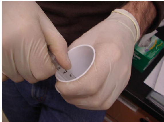
Fig. 14.23 Mixing of silicone base and curing agent
