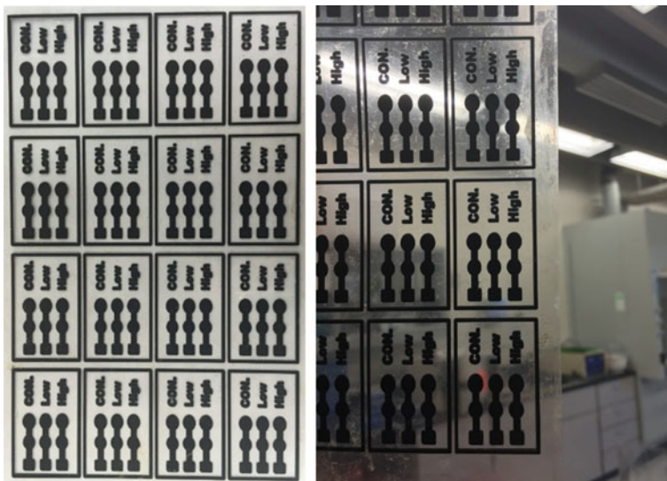
Fig. 14.29 A mask printed on a transparency film. Each LOC pattern consists of three keyhole-shaped straight channels, for a negative control (“CON”), and low- and high-concentration targets (“low” and “high”)
