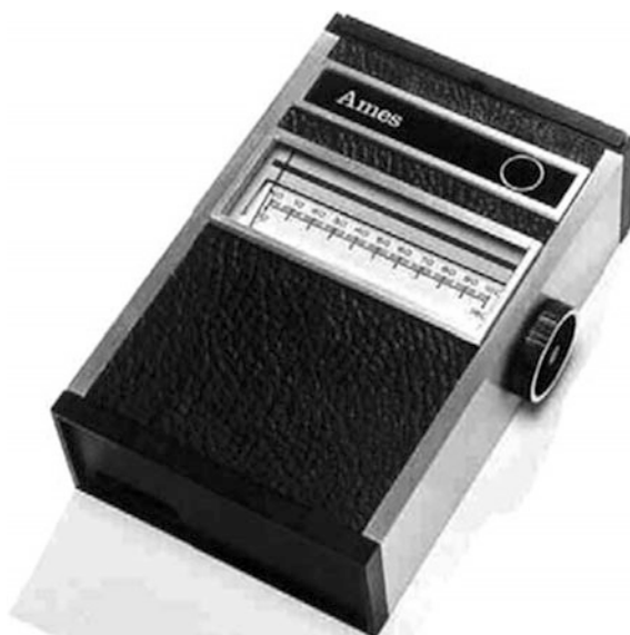
Fig. 12.1 Ames reflectance meter that reads from dextrostix. Reprinted from Newman & Turner. Biosens. Bioelectron. 20: 2435-2453, © Elsevier 2011, with permission from Elsevier
