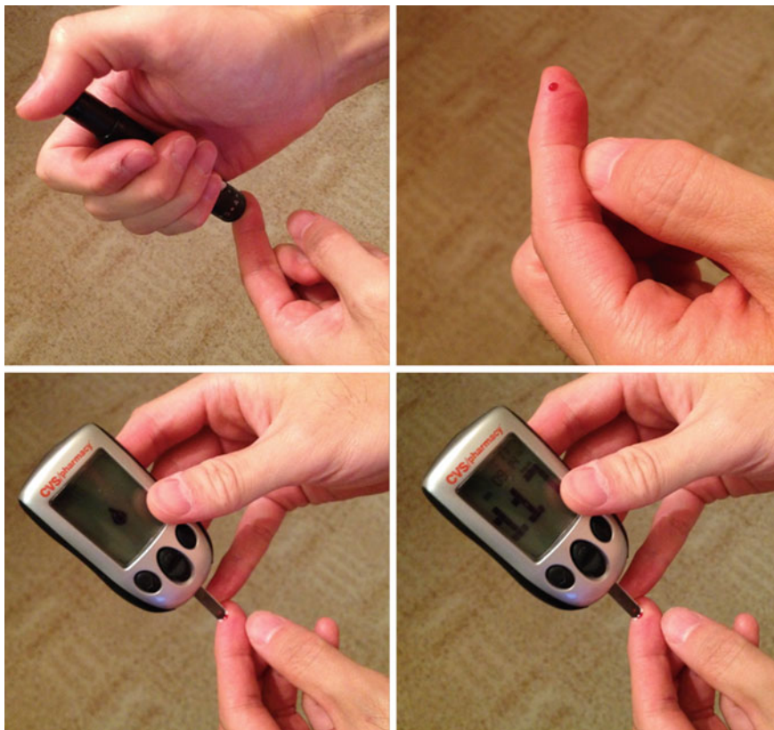
Fig. 1.9 A commercial glucose meter is reading the glucose level from blood, using an electrochemical transducer
