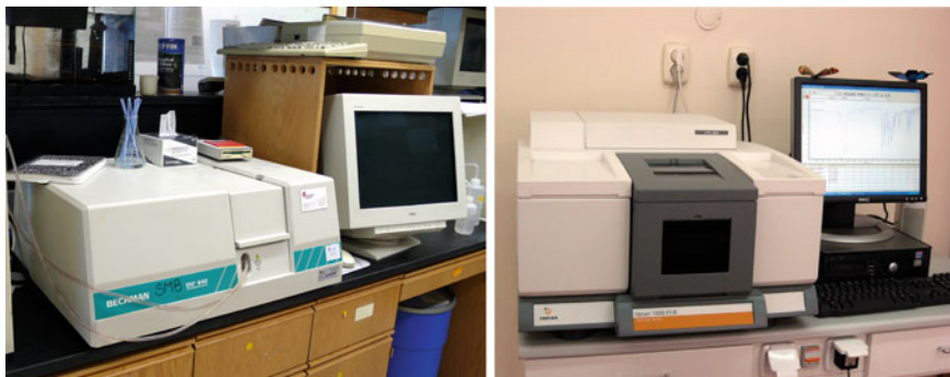
Fig. 8.1 Left a UV/Vis spectrophotometer. Right a FT-IR spectrophotometer. Pictures taken by Tim Vickers in July 2008 ( left ) and S. Levchenkov in June 2008 ( right ) and placed in public domain. Accessed October 2015 from http://commons.wikimedia.org/wiki/File:DU640_spectrophotometer.jpg ( left ) and http://commons.wikimedia.org/wiki/File:IR_spectrometer.jpg ( right )
