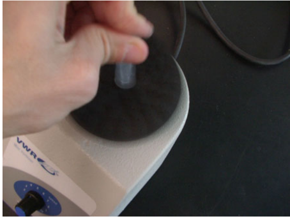
Fig. 8.16 A vortex mixer dissolving hemoglobin in a centrifuge tube
