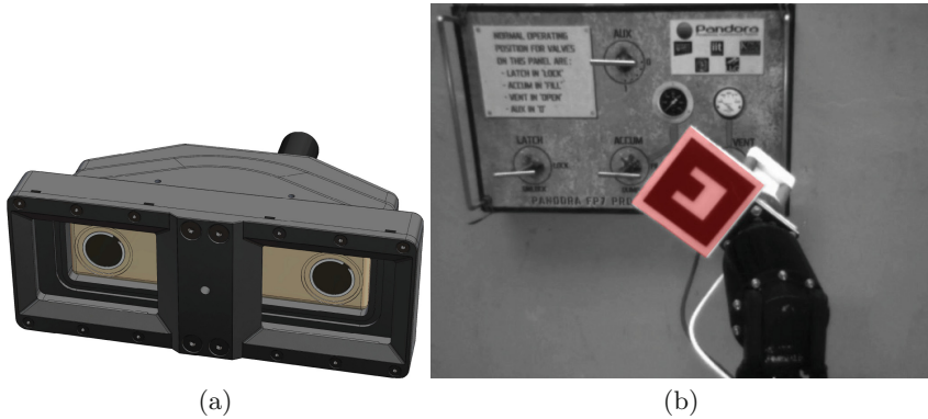
Fig. 3. (a) Stereo camera with housing. (b) ARToolkit algorithm detecting landmark mounted on the wrist of the manipulator.
