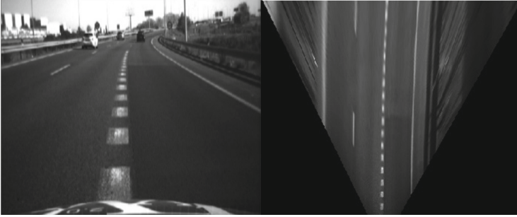
Fig. 2. Homography transformation from road image into bird view, right frame: ROI_{bv} (x_{bv}, y_{bv}, z_{bv}) .
