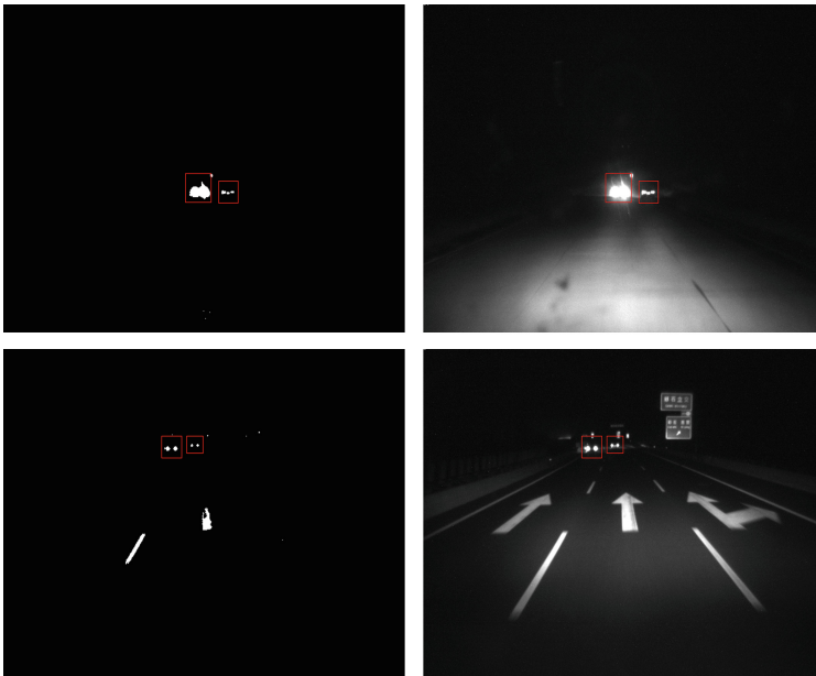
Fig. 5. Detection results. Top row: In pre-processed image from testing ground, and result marked in input image. Bottom row: In pre-processed image from highway, and result marked in input image
