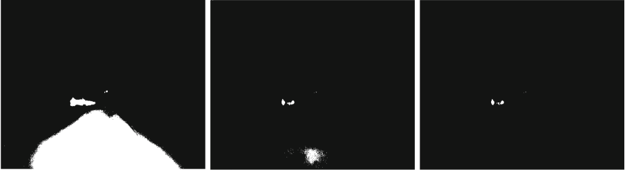
Fig. 4. Comparison of the three threshold methods. Left: Otsu's algorithm. Center: Kumar's method. Right: Our improved thresholding method
