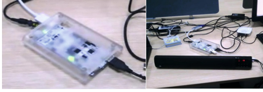
Fig. 7. Hardware implementation of a mobile speech emotion recognition system using pcDuino
