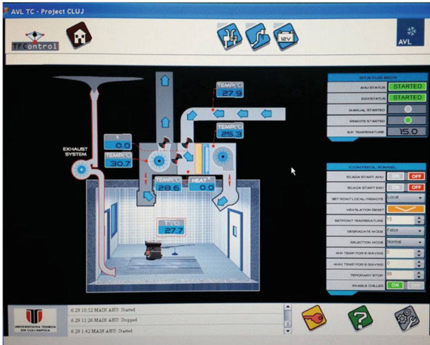
Fig. 3 Control interface of the conditioning system
