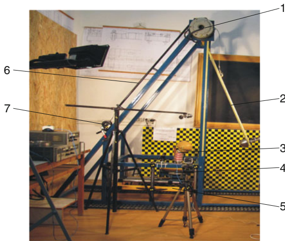
Fig. 7 Experimental stand with cranio-cervical classic system ready for testing : 1 electromagnetic brakes; 2 pendulum; 3 classic cranios-cervical system, 4 rotational system for cranio-cervical system; 5 vertical and horizontal translation system (3 axes); 6 guide cable; 7 position winch pendulum
