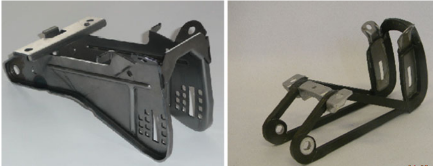
Fig. 11 Steering column bracket steel ( left ) and carbon fiber ( right )
