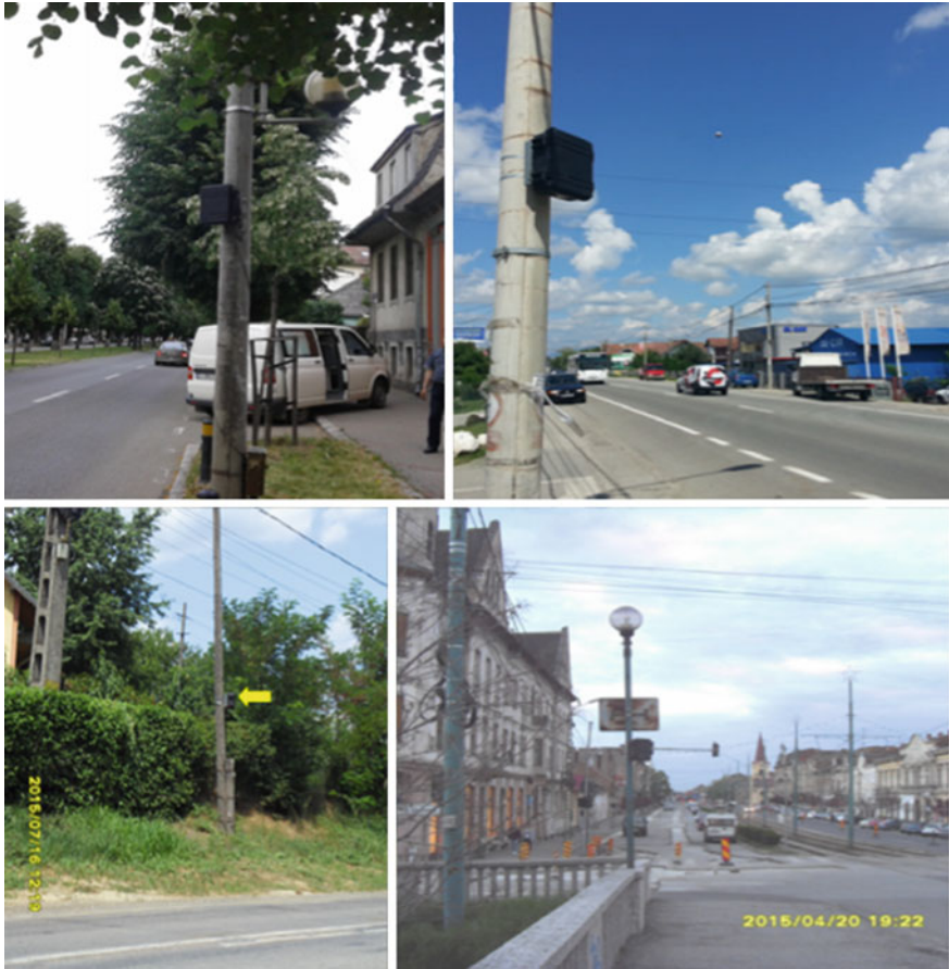
Fig. 1 Mobile traffic data count in different work conditions (Road traffic laboratory of UTCN projects for develop urban mobility plan in different cities from country)
