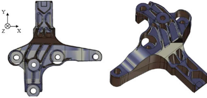
Fig. 2 The first numerical model of the engine mount
