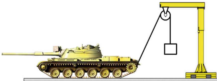
Fig. 2 Experimental rigging to evaluate a vehicle's transmission moments of inertia
