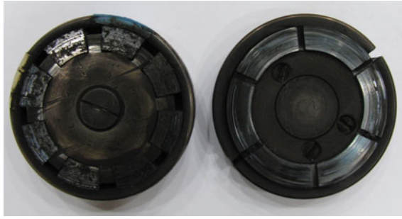
Fig. 2 Example of model friction pair used in IL-68 tests ( right friction material samples, left cast iron countersample)
