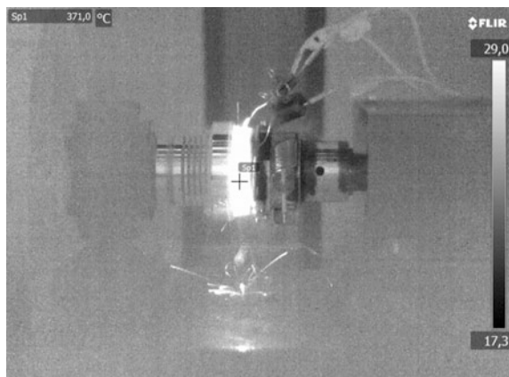
Fig. 4 Hot particles leaving friction contact during IL-68 test (sample frame from thermographic camera recording)
