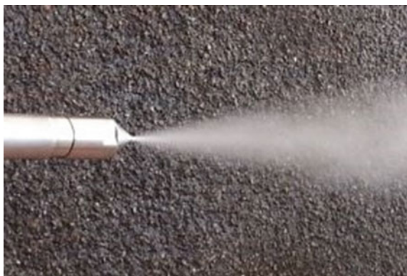
Fig. 16 Spray in free field, air-water injection system
