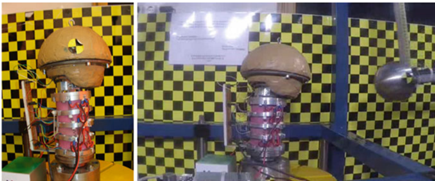
Fig. 8 The cranio-cervical artificial muscles biofidelity driven based on shape memory springs ready for experimental testing
