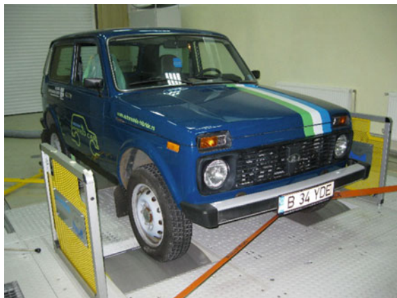
Fig. 1 Small off-road vehicle with prototype hybrid powertrain developed at the automotive engineering department of the university POLITEHNICA of Bucharest
