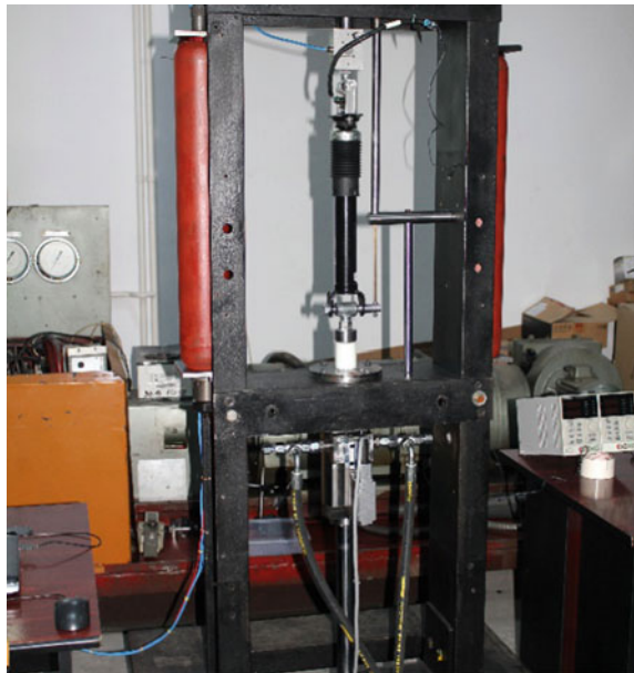
Fig. 1 The frame of the test bench for shock absorbers
