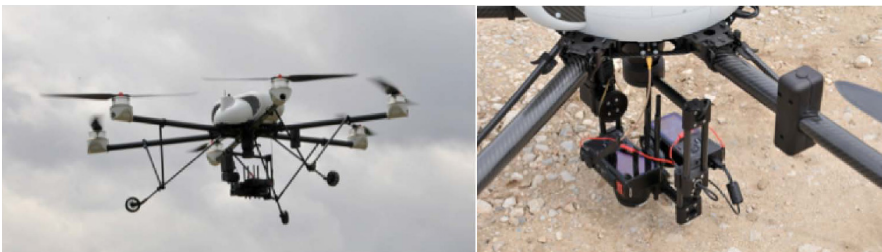
Fig. 2 AR200 drone in flight with a detail of the camera mounting
