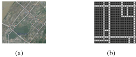
Fig. 4. The area centering Xudong in Wuhan (a) from Google maps is mapped to lattice space (b) in EBML. The white lattices denote the roads. The black lattices denote the blocks. The gray lattices denote intersections.
