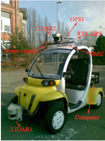
Fig. 5. Experimental vehicle equipped with sensors (camera and RTK-GPS)
