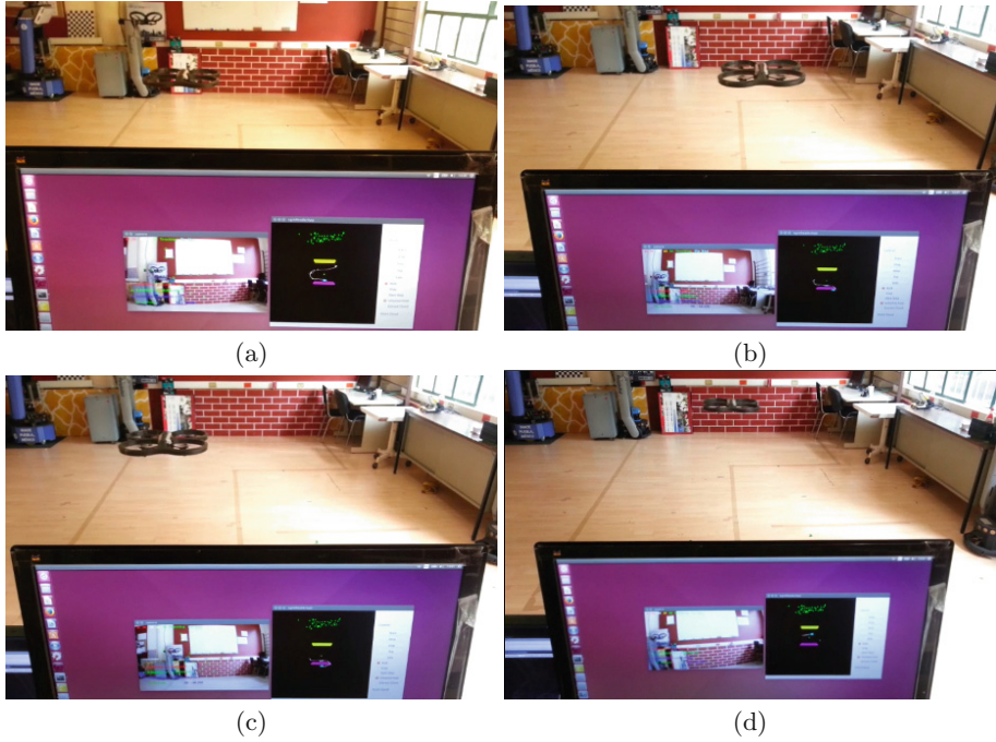
Fig. 5. Snapshots of a representative run with the order (a,b,c,d), the vehicle flies autonomously driven by the PD controller that uses our visual odometry approach to calculate the corresponding control signals.
