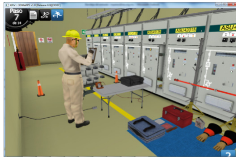
Fig. 3. Performing the electrical tests for metal clad switchboards.
