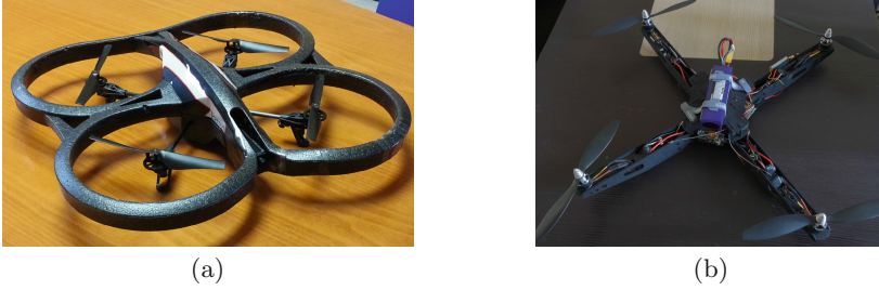
Fig. 1. Micro Aerial Vehicles used in this work: (a) commercial quadcopter AR Drone; (b) custom-built quadcopter.
