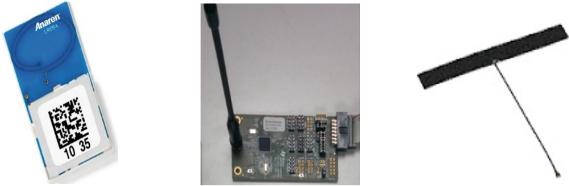
(a) SN with low gain antenna (b) SN with high gain antenna (c) WUR bendable antenna
