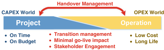
Fig. 1 CAPEX to OPEX transition incorporating handover management
