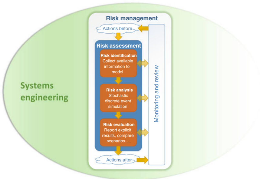
Fig. 1 Risk assessment process as a part of risk management and systems engineering
