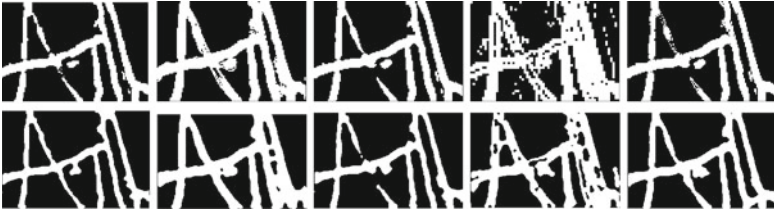
Fig. 4. Final result of the segmentation algorithm for SEM images. First row represents the outputs of the artificial neural network for the Experiments I, II, III, IV and V. Second row represents the results of the postprocessing step corresponding to the output of the artificial neural net (first row).
