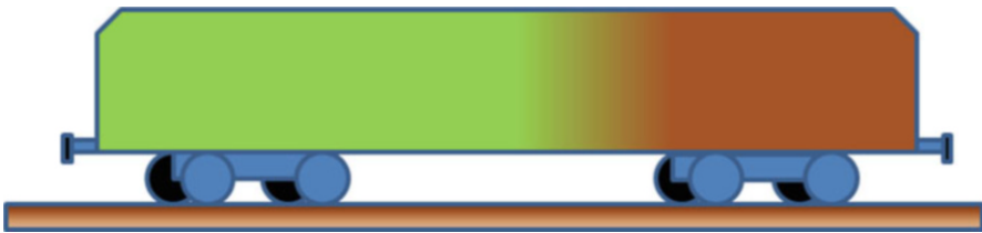
Fig. 4.4 A standard wagon with four sets of wheels
