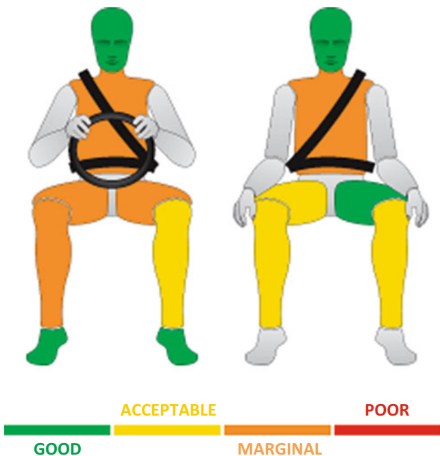
Fig. 1.5 Common injuries for the driver and passenger in ANCAP 4 Star (Australian NCAP 2012)
