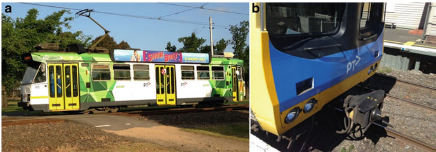
Fig. 4.3 (a) A single wagon as an example for basic tram/train elements modeling; (b) Connection interface that will be modeled as a spring
