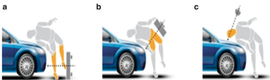
Fig. 1.10 Subsystem test for Pedestrian Protection in Euro NCAP (Euro NCAP 2012) (a) Leg form (b) Upper leg form (c) Head form
