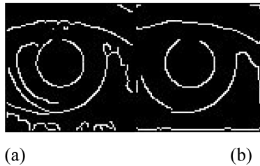
Fig. 8. Comparison between the results of edge detecting. (a) is the result without Gaussian filter processing. (b) is the result with Gaussian filter processing.
