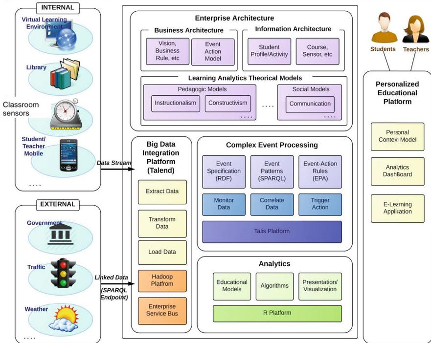
Fig. 1. Example of smart university platform
