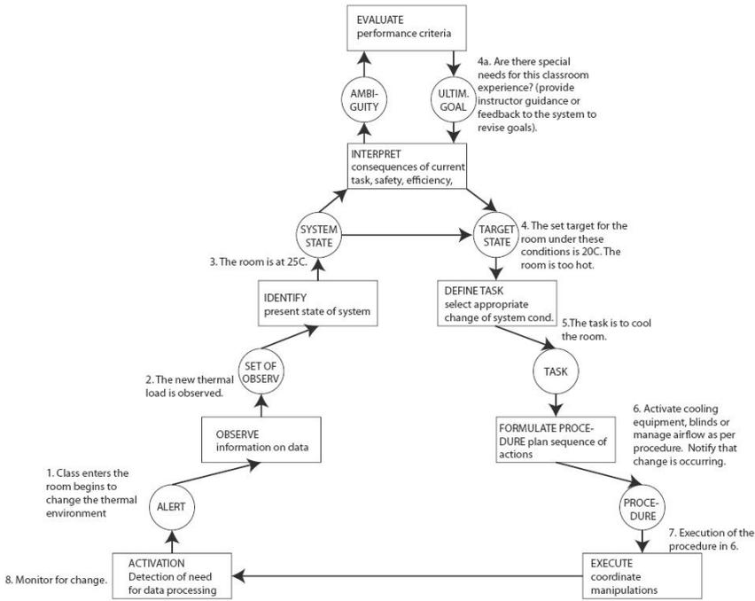
Fig. 3. Monitoring room temperature in the smart campus scenario.
