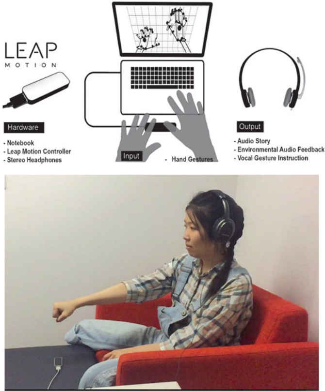
Fig. 1. Experiment setup: hand motion input, processing, and audio output
