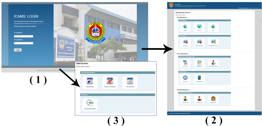
Fig. 3 User is requested to login at the index page (1) before they can access to the home page (2) of the system. Features that are available to the user changes accordingly to the user's account type. The administrator accounts are allowed to adjust various system settings and configurations, and perform administrative management. The staff accounts (3) are essential for schedule management. Attendance tracking for whole class and individual student are accessible by both staff and student accounts respectively.
