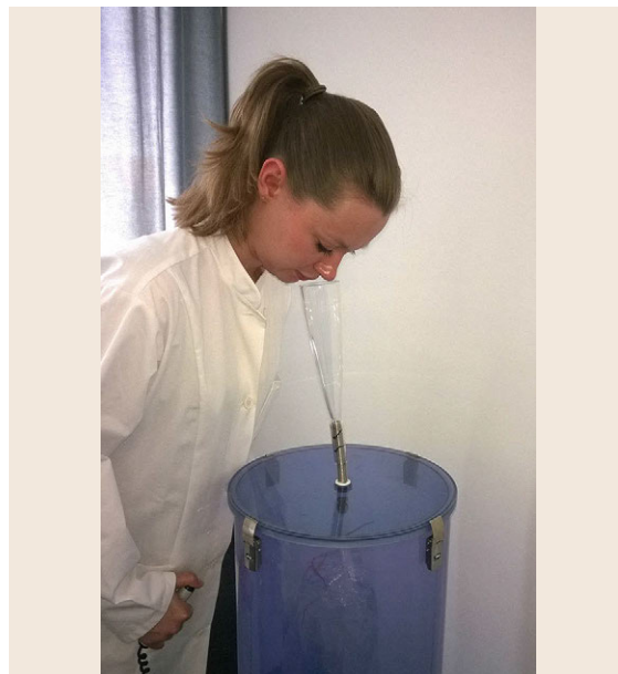
Fig. 26.10 A panelist evaluates an air sample provided by controlled deflation of an air sampling bag using a direct sniffing system (PureSniff) (courtesy of Fraunhofer IBP)
