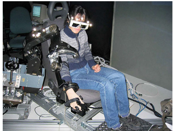
Fig. 55.5 Haptic feedback by an exoskeleton device (courtesy of Fraunhofer IAO, University of Stuttgart IAT)
