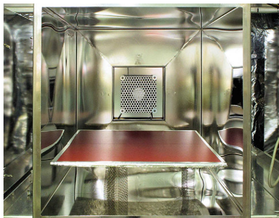
Fig. 26.7 Floor sample in a 200 l emission test chamber (courtesy of Fraunhofer IBP)
