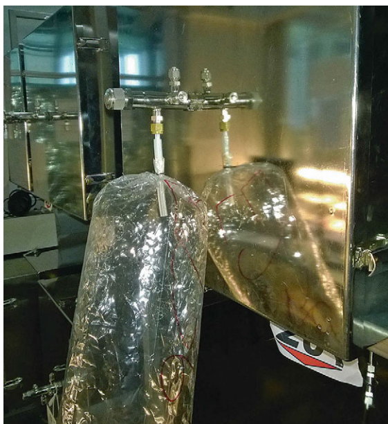
Fig. 26.9 Sampling of air from an emission test chamber into a sampling bag for subsequent odor evaluation (courtesy of Fraunhofer IBP)
