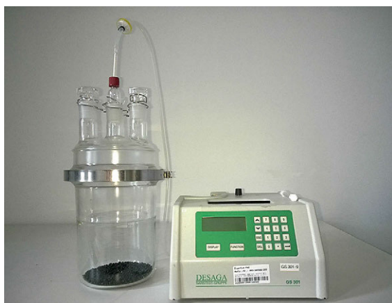
Fig. 26.6 Sampling of emissions from polymer granules for GC-O analysis. The sample is placed in a gas-tight headspace vessel. A pump sucks air through a small tube filled with Tenax TA adsorbent material (courtesy of Fraunhofer IBP)
