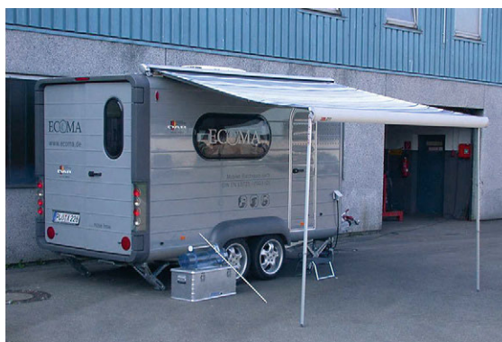
Fig. 24.3 Mobile measurement laboratory (odor room) in use on site
