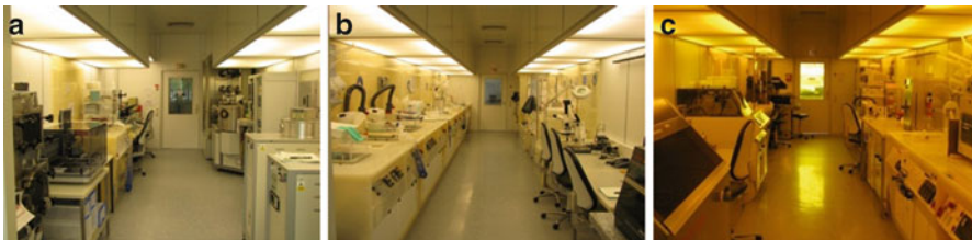
Fig. 2.2 The three “white” cleanroom corridors in the Institute of Microtechnology at TU Braunschweig: (a) process unit aisle; (b) area of chemical processing and (c) yellow-light aisle for photolithography
