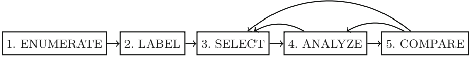
Fig. 1. Our workflow starts with the enumeration (1) of all possible parametrizations that fit the expectations of the modeller about the structure. Each of the parametrizations is evaluated for certain properties (2) like dynamical behaviour, and the result of the evaluation is stored with the parametrization as its label . After parametrizations are labelled the user can select (3) a subset of these that seem of special interest. This selection can then be analysed using various tools (4) and compared to other selections (5). The selection or analysis can then be refined based on the newly gained knowledge.
