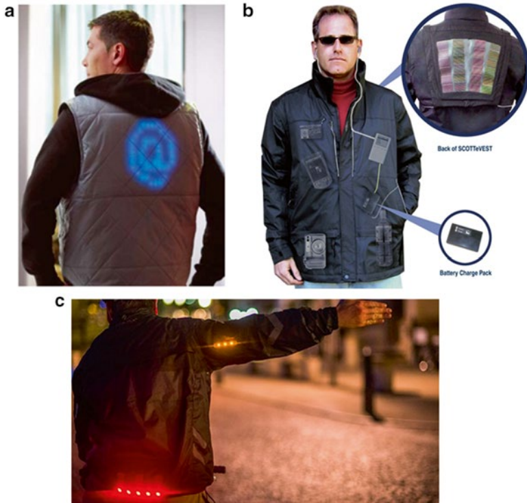
Fig. 6.6 Functionalized smart jackets: (a) Philips Lumalive LED-based jacket, with permission from [109]; (b) Scottevest Solar Jacket with added functionality, with permission from [107]; and (c) Visijax commuter jacket with turn signals, uses Eleksen’s conductive textile technology, with permission from [136]
