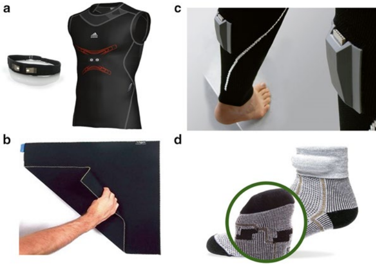
Fig. 6.5 Health and sports applications of textile sensors: (a) NuMetrex heart rate monitoring shirt and chest strap, with permission from [83]; (b) Sensing Tex textile system for measuring pressure distribution, with permission from [84]; (c) ESA muscle monitoring suit for astronauts, by Ohmatex, with permission from [69]; and (d) Sensoria smart sock for foot pressure measurements, with permission from [85]
