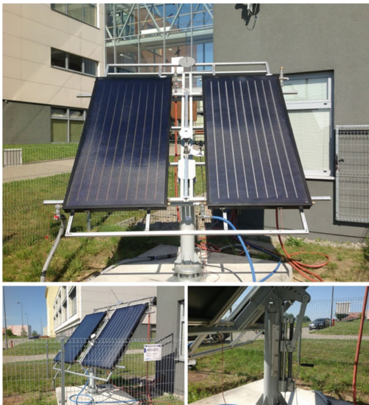
Fig. 9 Outdoor solar collector experimental setup
