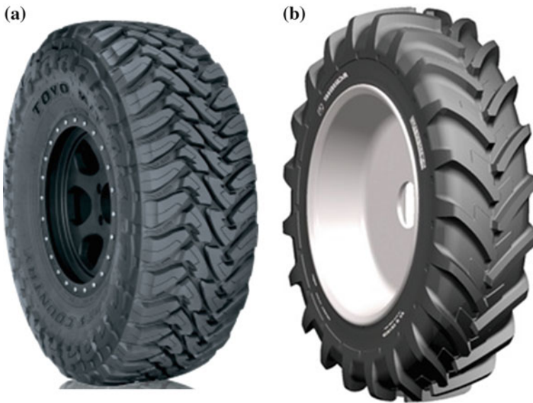
Fig. 5 Examples of off-road tires for conventional vehicles: a Open Country M/T sport utility vehicle tire—Toyo [15], b Agribib tractor Tire—Michelin [16] (sizes are not to scale)
