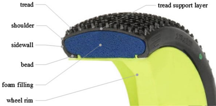
Fig. 6 Cross section of a non-pneumatic tire of the type used in the lightweight wheeled mobile robots (source of the background image: Pro-Line racing [17])
