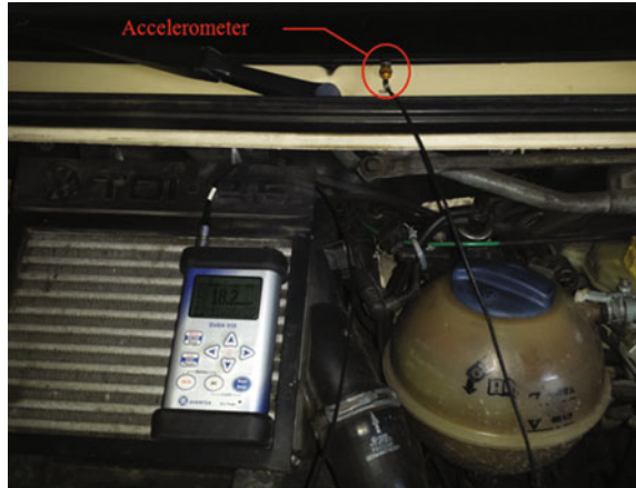
Fig. 16 Location vibration measuring system for the P2 measurement point
