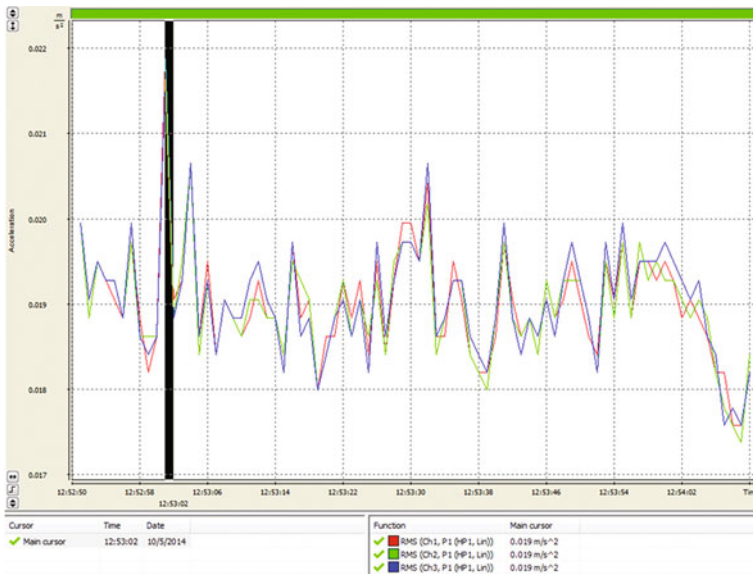
Fig. 15 Oscillogram of RMS acceleration from the P1 measuring point
