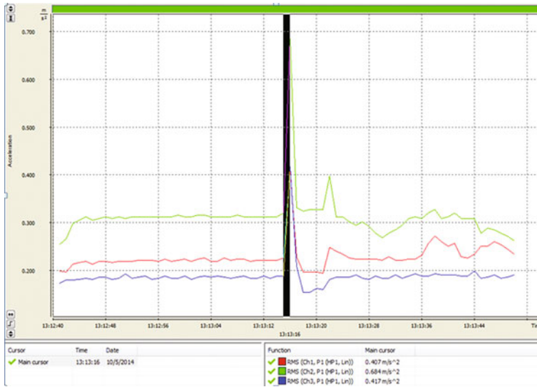
Fig. 21 Oscillogram of RMS acceleration from the P3 measuring point
