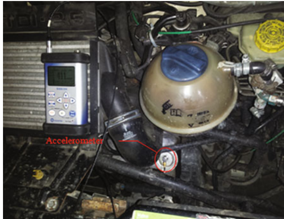
Fig. 13 Location vibration measuring system for the P1 measurement point
