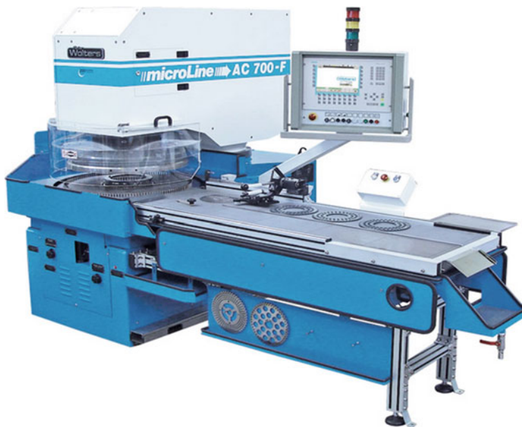
Fig. 2 Lapping machine with feeding table [15]
