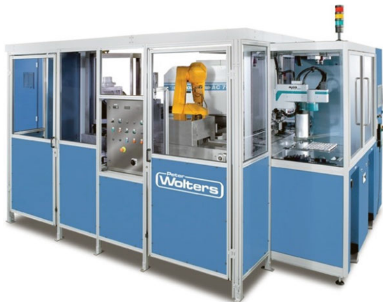
Fig. 3 Robot as a feeder in Peter Wolters lapping machine [15]
