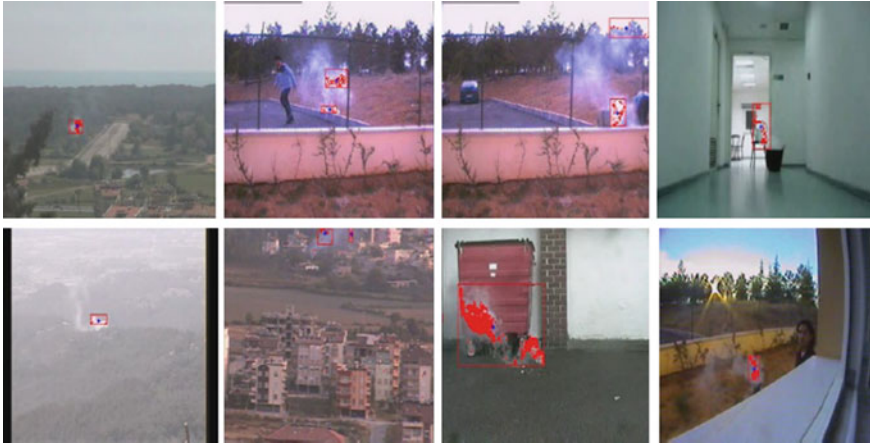
Fig. 18 Experiment 2 results from the videos with smoke processed with the proposed method
