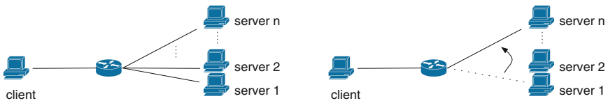
(a) SDN-multicast transparently forks TCP flows to n servers in separate datacentres, allowing for data replication in real time
