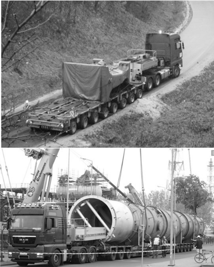
Fig. 5 Example of special vehicle used in oversized cargo transportation (source: [26])
