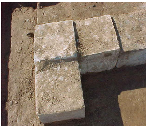
Fig. 9.8 Blocks of cemented waste in an opened experimental repository after 40 years of burial ( Source: Sobolev et al. [63] )
