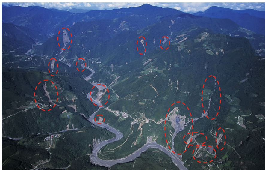
Fig. 10.1 Photo showing extensive landslides in the catchment of the Shihmen Reservoir during Typhoon Aere in 2004
