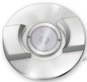
Fig. 7.2 Makler counting chamber. [Reprinted with permission, Cleveland Clinic Center for Medical Art & Photography © 2015. All Rights Reserved.]
