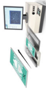
Figure 5. Correct loading of a counting chamber into the CASA analyzer.
