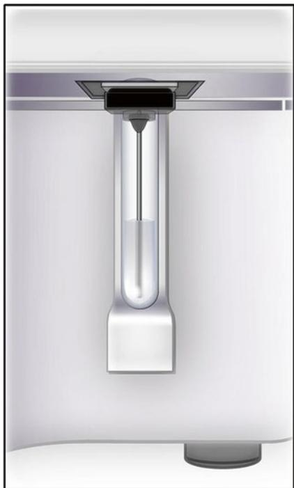
**Fig. 24.11** Tube filled with 0.22  $\mu\text{m}$  DI water placed on SIP [Reprinted with permission, Cleveland Clinic Center for Medical Art & Photography © 2015. All Rights Reserved]
