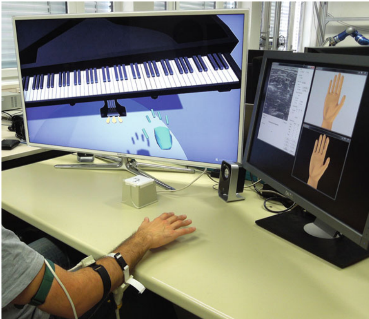
Fig. 11.1 The setup used in [11]. A magnetic tracker and an ultrasound transducer are fixed on the subject's forearm; an HMI based upon iRR converts local spatial features of the ultrasound images to finger forces (screen on the right ); lastly, finger forces and wrist position are used in a virtual setup (screen on the left ) to play a piano
