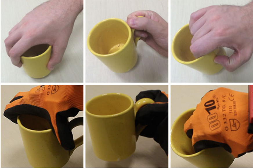
Fig. 8.15 A human hand grasping a cup with three different approaches ( top panels ) and the same grasps reproduced with the Pisa/IIT SoftHand ( bottom panels )
