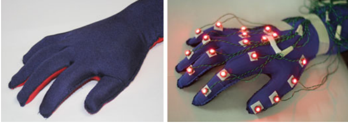
Fig. 15.3 The sensing glove used in our study ( on the left ) and the sensing glove with added markers ( on the right )
