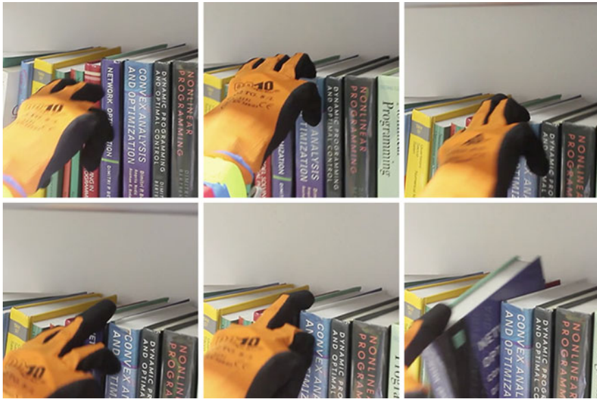
Fig. 8.17 A person with the arm-mounted SoftHand can seamlessly execute also difficult manipulation tasks which involve combined interactions between hand, object and environment
