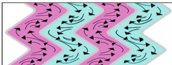
Fig. 4 Flow patterns in corrugations of plate heat exchanger (With permission from HTRI)
