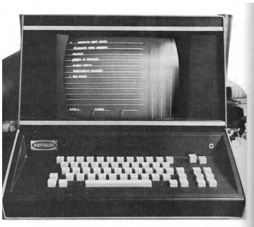
Fig. 2. The homemade touch-screen interface to an interactive display terminal used for progress note entry in 1969 hypertension progress note structured data capture project. See [10].
