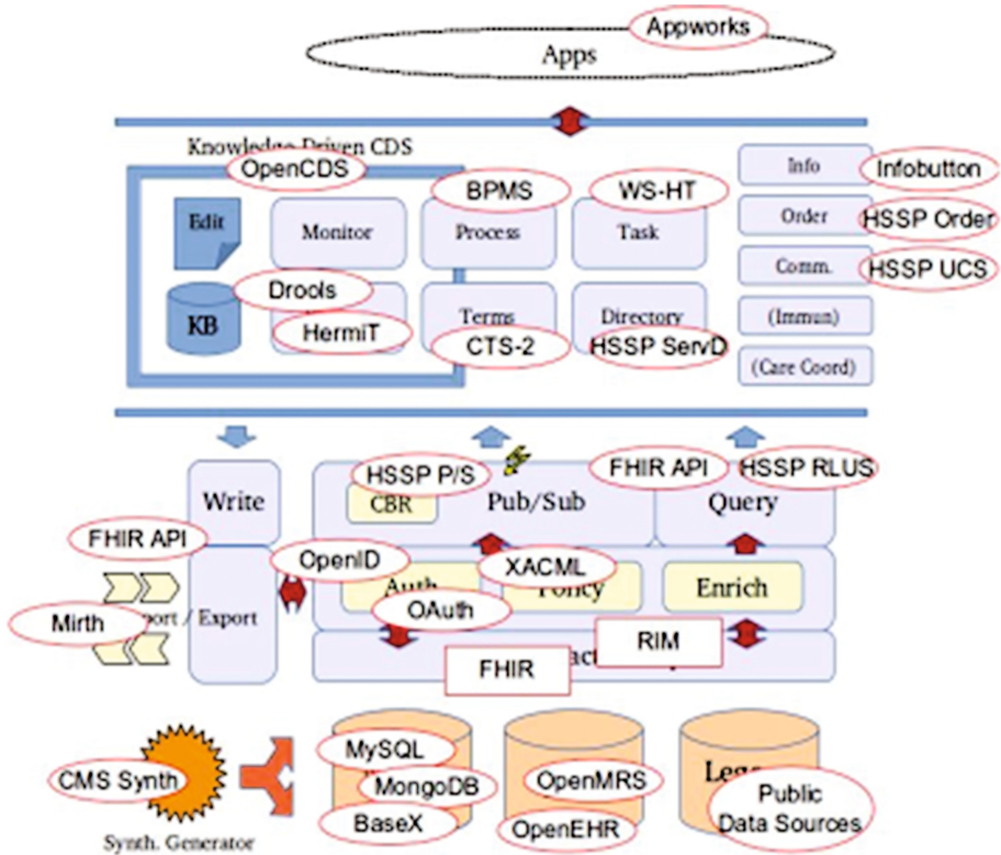
Fig. 7. A multi-tiered standards-based architecture being developed for supporting apps and suites of apps operating on top of multiple data sources including EHRs. This indicates the intermediate tier services that are assembled to provide the platform. Classes of services are shown with candidate particular services indicated. (Adapted from [39] with permission, and modified courtesy of D. Sottara, Arizona State University).
