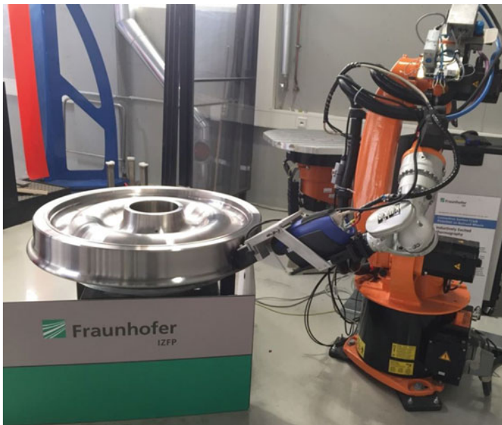
Fig. 16 Demonstrator set-up for surface defect testing on railway wheels by induction thermography using a robot
