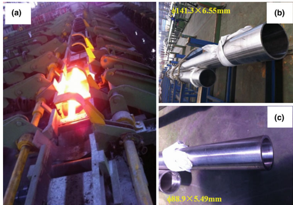
Fig. 8 Hot extrusion of alloy pipes: a hot extrusion process, b \phi = 141.3 mm pipe, c \phi = 88.93 mm pipe
