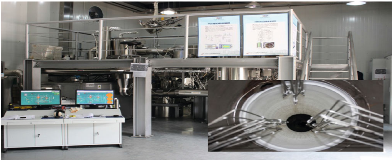
Fig. 5 Picture of frozen-wall facility and image of the formed frozen wall ( Inset )
