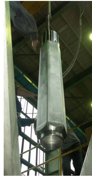
Fig. 2 Manipulation with the salt zone before insertion into reactor core
