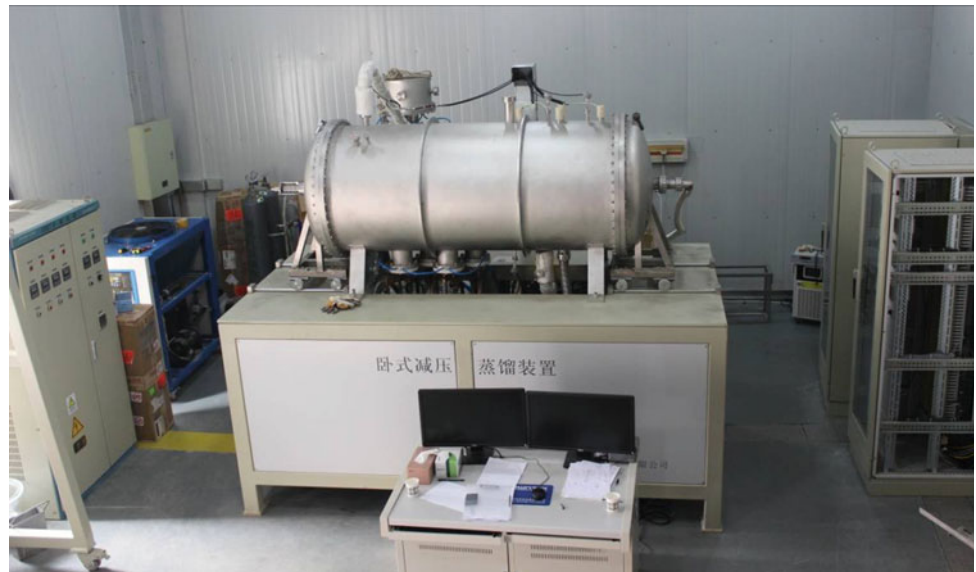
Fig. 6 Picture of the horizontal distillation facility
