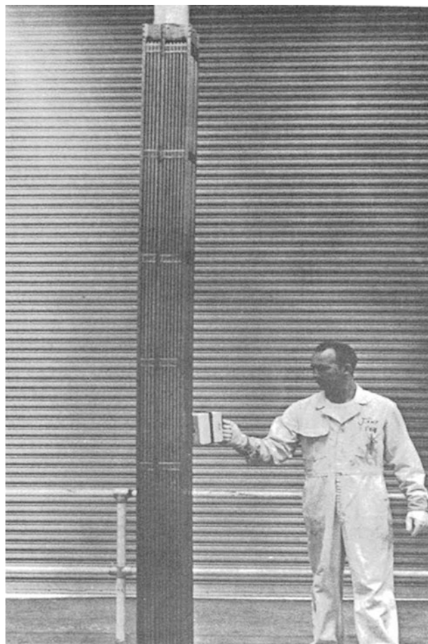
Fig. 2 Finished fuel assembly produced during demonstration program (withdrawn rapidly from pool for quick survey of gamma activity)
