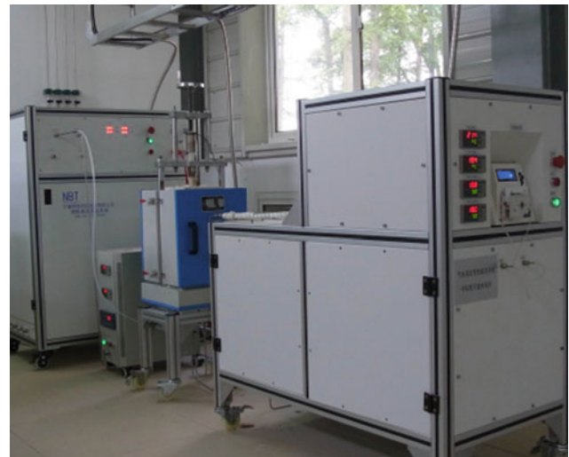
Fig. 10 kW integrated SOEC evaluation platform
