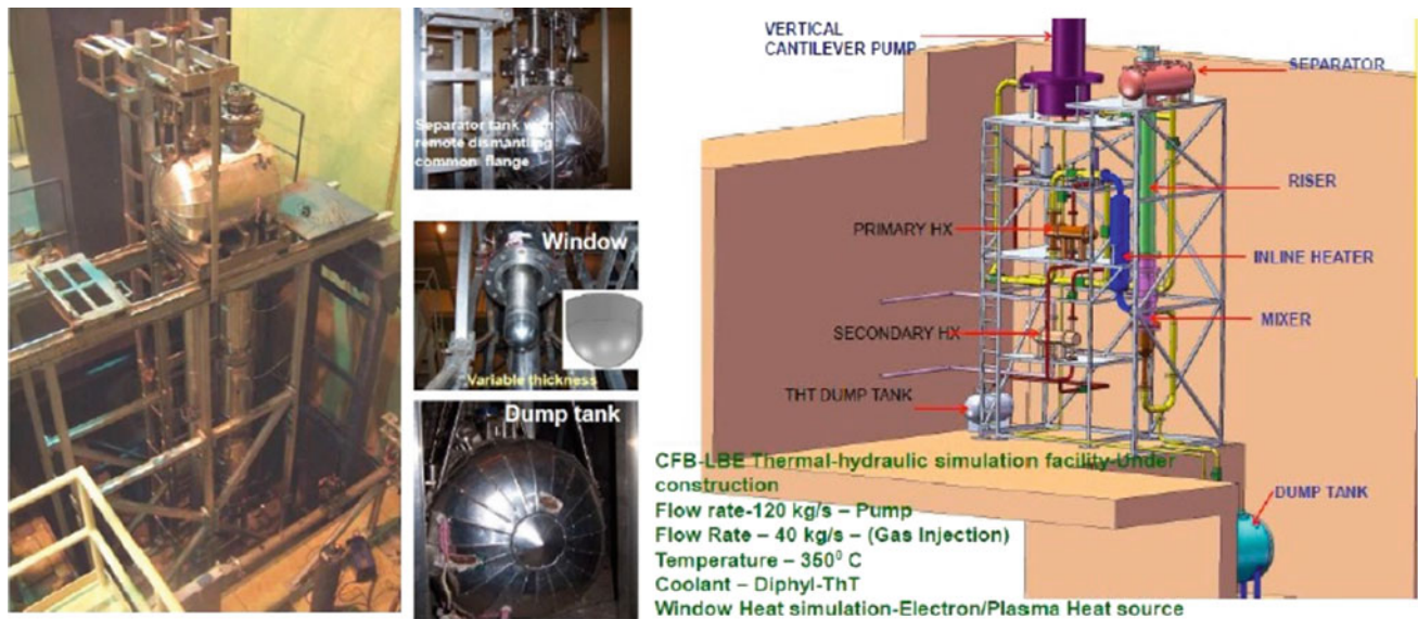
Fig. 2 Left Various components of the target to be irradiated in the medical cyclotron, VECC, Calcutta. Right LBE loop coming up at Trombay
