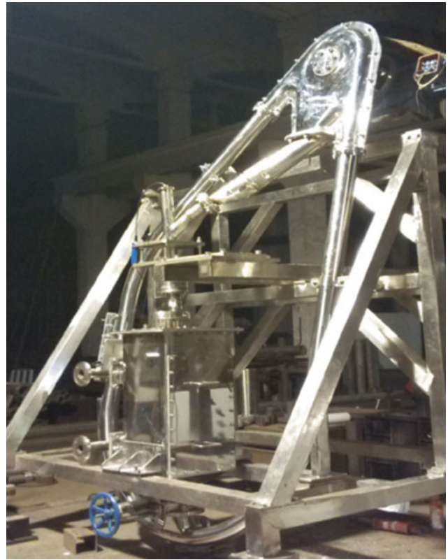
Fig. 3 A small-scale test system of the DGT, including the beam interaction chamber, the heat exchanger, the pipe chain elevator and so on
