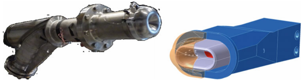
Fig. 2 Tested Eurisol target ( left ) and derived T-MIF target concept ( right )
