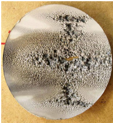
Fig. 5 SNS beam window inner surface sample extracted after irradiation
